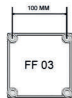
FF 03 HEIGHT: 120 MM Leave 35 MM from top of nut to finished concrete level
