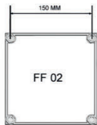
FF 02 HEIGHT: 200 MM Leave 45 MM from top of nut to finished concrete level
