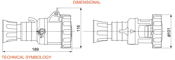
IP IK 166/IP67/IP68/IP69 IK09 -25 +55 °C With screw With screw Halogen-free in compliance with EN -650 °C (active parts) 125 °C (active parts) -80 °C (passive parts) -80 °C (passive parts)
